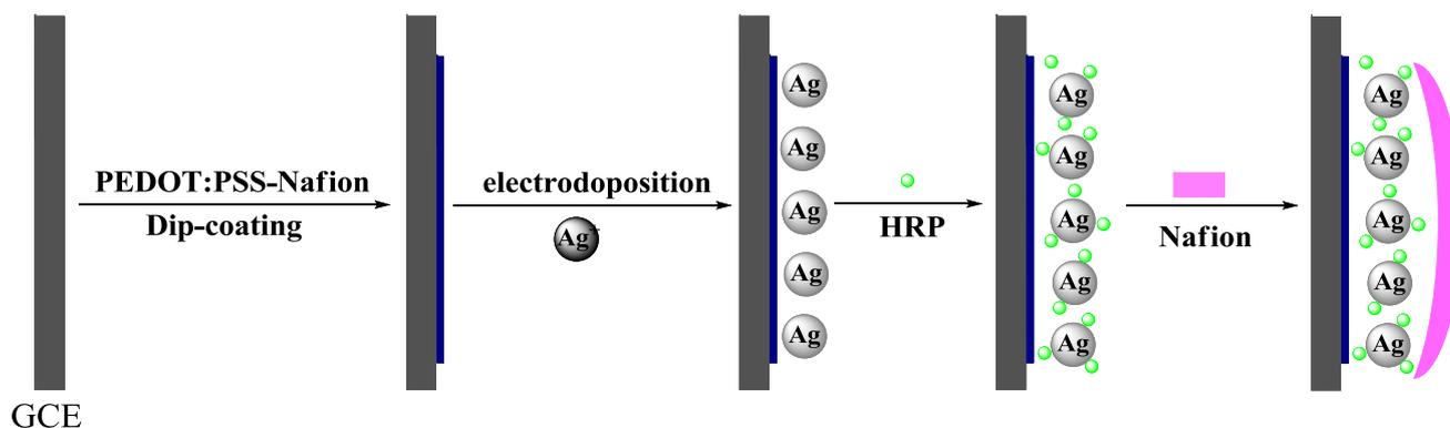
**Scheme 1.** Preparation process of Nafion/HRP/AgNPs/PEDOT:PSS-Nafion/GCE composite electrode.
