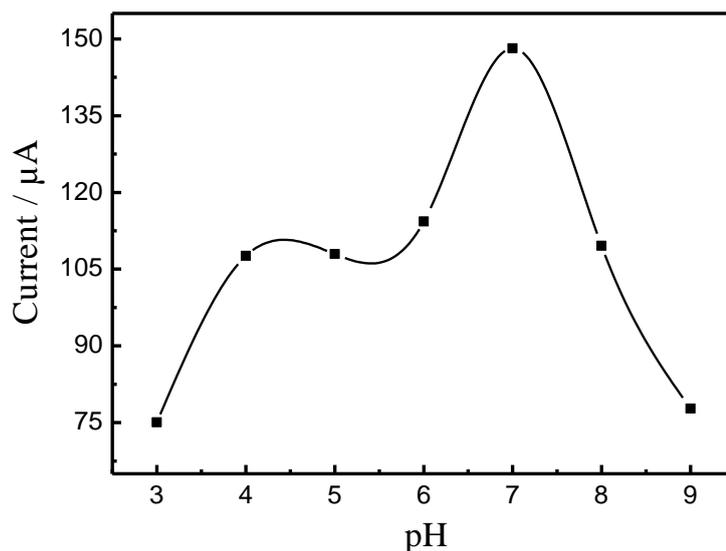
**Figure 5.** Effect of pH on the oxidation peak currents of Nafion/AgNPs/HRP/PEDOT:PSS-Nafion/GCE in 0.1 M PBS (pH 7.0) containing 40  $\mu\text{M}$   $\text{H}_2\text{O}_2$ . Scan rate: 50  $\text{mV s}^{-1}$ .
