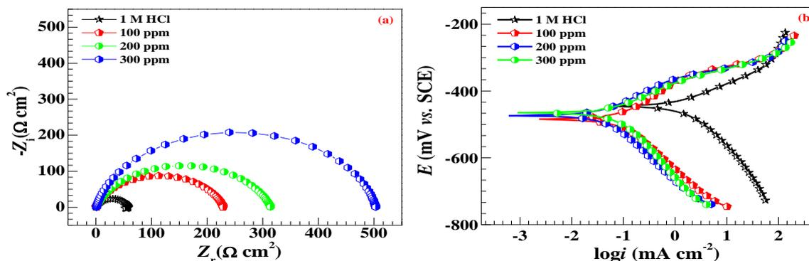
**Figure 2.** (a) Nyquist plots in absence and presence of different concentration of Cephamycin and (b) potentiodynamic polarization curves in absence and presence of Cephamycin
