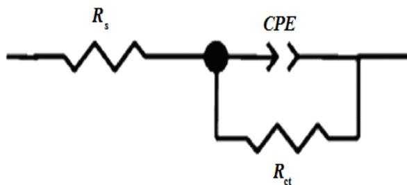
**Figure 3.** electrochemical equivalent circuit used to fit the impedance measurements that include a solution resistance ( $R_s$ ), a constant phase element ( $CPE$ ) and a polarization resistance or charge transfer ( $R_{ct}$ )
