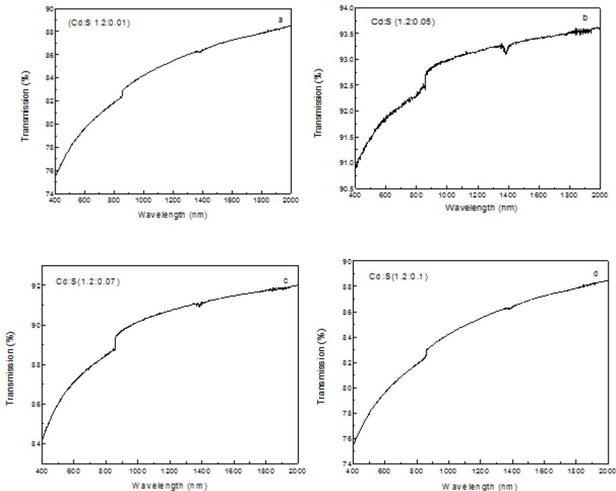
**Figure 4.** Transmission (%) of CdS nanostructures at different thiourea concentrations 0.01 (a), 0.05 (b), 0.07 (c) and 0.1 (d) mol/L
