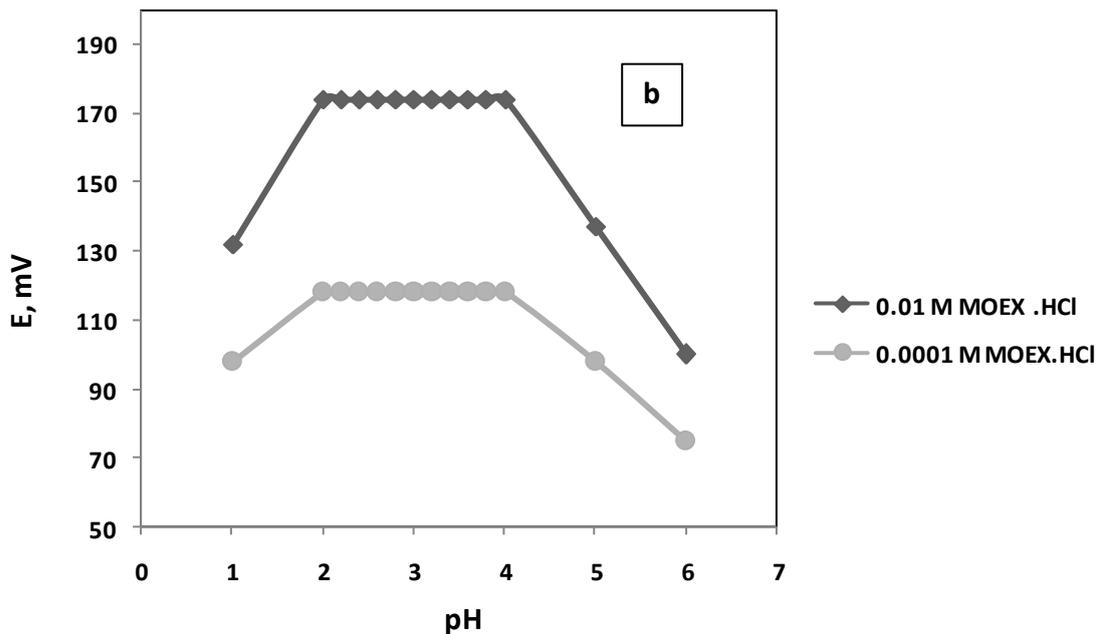
**Figure 3.** Effect of pH on the electrodes performance using (a) CPE and (b) PVC membrane potentiometric sensors.
