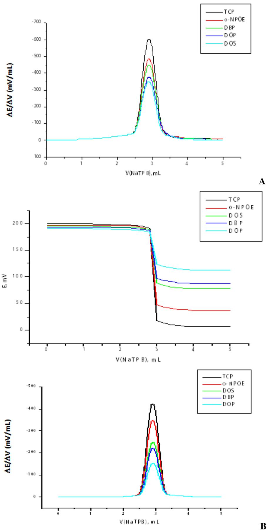
Figure 4. The effect of plasticizer type using: a) CPE and b) PVC membrane electrodes.
