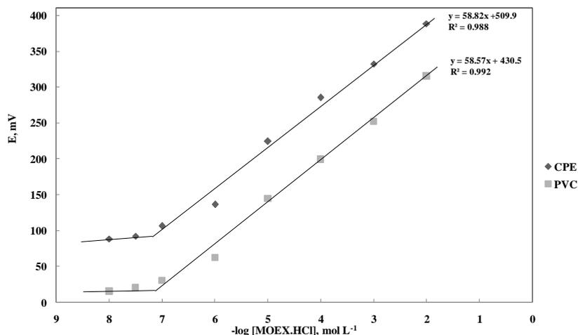
Figure 2. Nernstian slope using CPE and PVC membrane potentiometric sensors.
