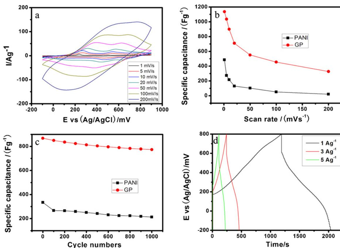
**Figure 1.** (a) Cyclic voltammety curves of GO/PANI composite at different scan rates (b) The specific capacitance value of GO/PANI composite and PANI recorded at different scan rates (c) Cyclic stability of GO/PANI composite and PANI electrodes measured at the current density of  $1.5 \text{ Ag}^{-1}$  and (d) charge-discharge curve recorded at different current densities ( $1 \text{ Ag}^{-1}$ ,  $3 \text{ Ag}^{-1}$  and  $5 \text{ Ag}^{-1}$ ) (Reproduced with permission from ref. [28]).
