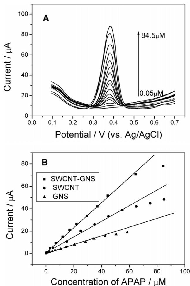
**Figure 5.** (A) DPVs at the SWCNT-GNS/GCE towards determination of acetaminophen at different concentrations of acetaminophen in 0.1 M phosphate buffer (pH = 7). (B) The corresponding calibration curves for acetaminophen at different electrodes (Reproduced with permission from ref. [67]).
