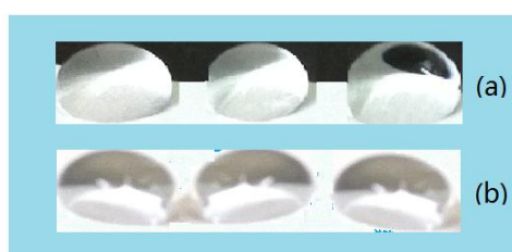
Figure 3. Results of Temperature on PTFE film contact angle influence, (a) PTFE film contact angle at room temperature, (b) PTFE film contact angle after boiling water immersion.
