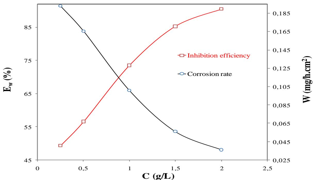
**Figure 1.** Variation of corrosion rate ( $W$ ) and inhibition efficiency ( $E_w$ ) of corrosion of mild steel in 1 M HCl with different concentration of *S. inaequidens* essential oil.
