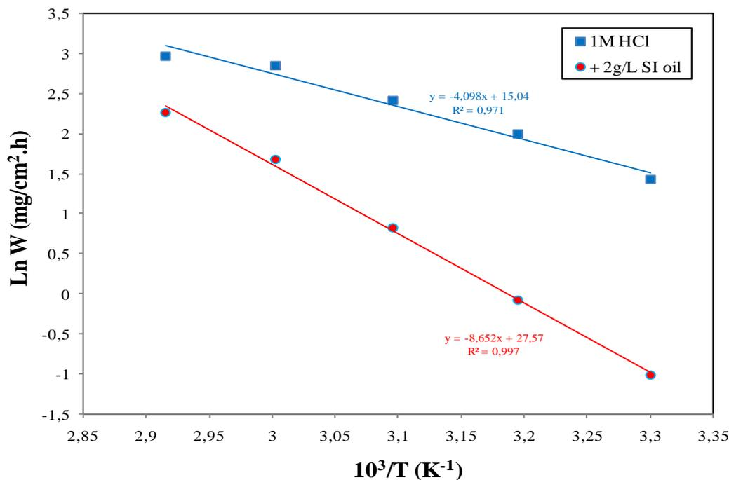
**Figure 3.** Arrhenius plots for mild steel corrosion rates ( $W$ ) in 1 M HCl in absence and in presence of 2 g/L of *S. inaequidens* oil.
