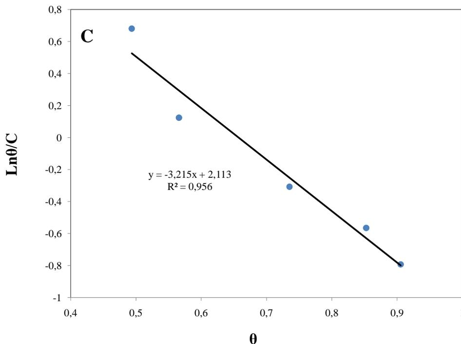
**Figure 5.** (A) Langmuir, (B) Frumkin and (C) Temkin isotherm for the adsorption of *S. inaequidens* essential oil on the surface of mild steel in 1 M HCl.
