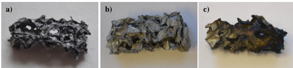
Figure 1. Carbonyl iron based cellular material prepared by powder metallurgy: Fe (a); Fe-CNTs (b); Fe-Mg (c). Sample diameter is 0.9 - 1 cm and length is 3.5 – 4 cm.
