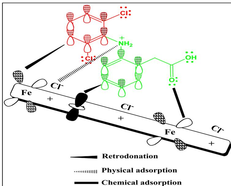
**Figure 11.** Mechanism of inhibition
