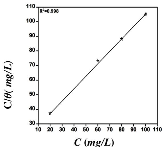
**Figure 6.** Langmuir's isotherm for adsorption of DS on mild steel surface in 1 M HCl
