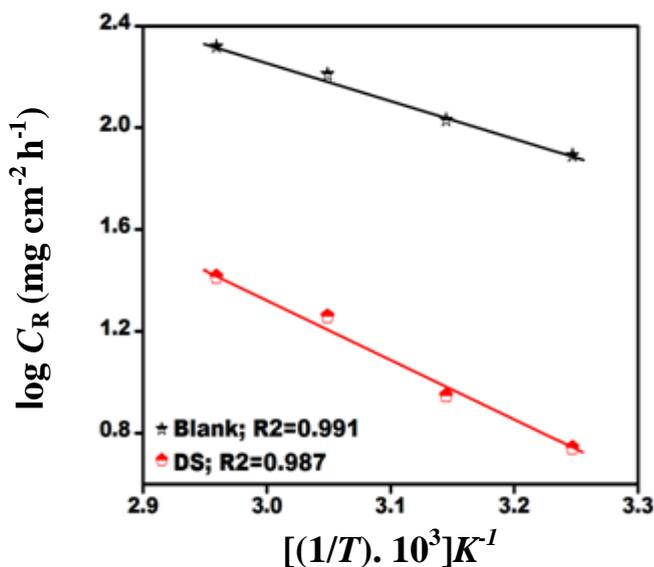
Figure 4. Arrhenius plot of mild steel in 1M HCl in absence and presence of different concentration of DS
