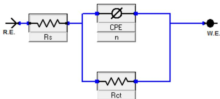
**Figure 8.** Equivalent circuit used to fit the EIS data
