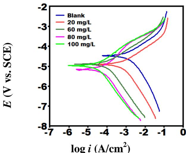
**Figure 10.** Potentiodynamic polarization curves for mild steel in 1 M HCl in absence and presence of various concentrations of DS at 308 K
