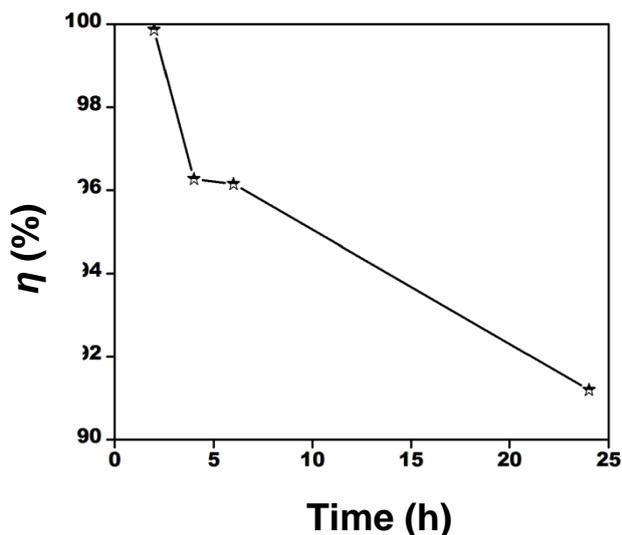
Figure 3. Variation of inhibition efficiency with Time
