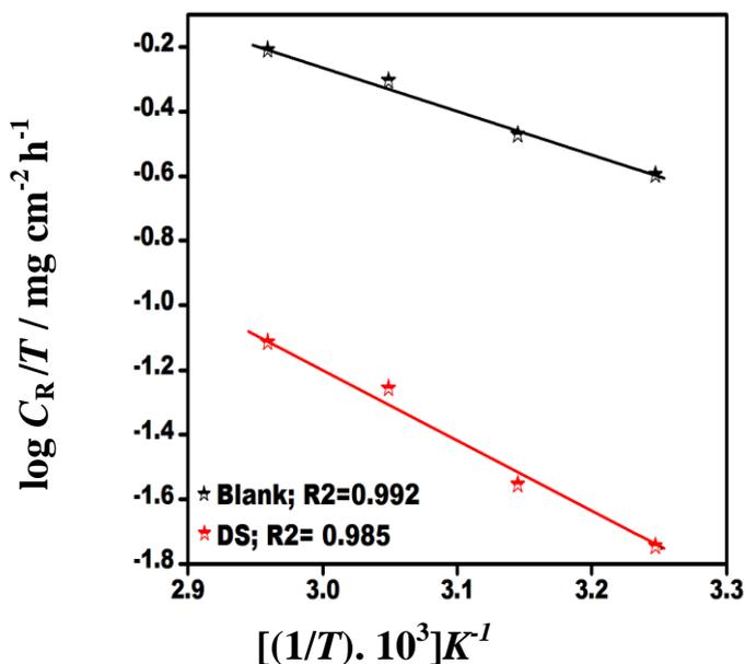
**Figure 5.** Transition-state plot of mild steel in 1 M HCl in absence and presence of optimum concentration of DS
