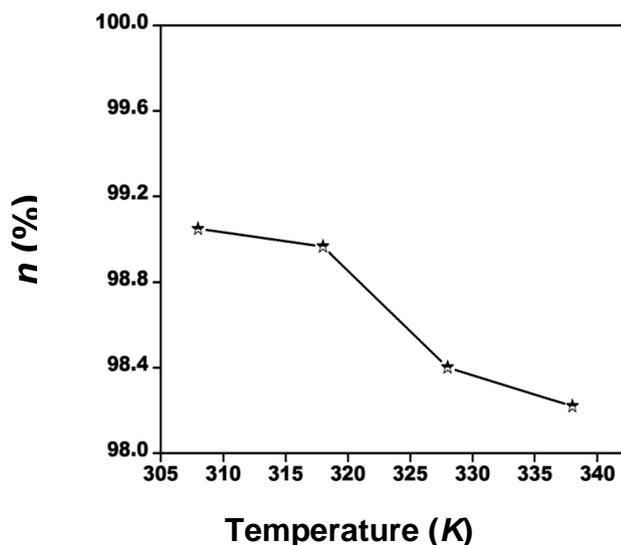
**Figure 2.** Variation of inhibition efficiency with Temperature
