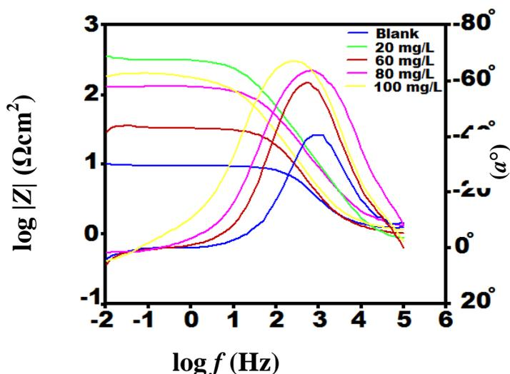
**Figure 9.** Bode impedance plots for mild steel in 1 M HCl in absence and presence of various concentrations of DS at 308K
