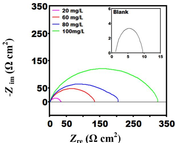
**Figure 7.** Nyquist plots for mild steel in 1 M HCl in absence and presence of various concentrations of DS at 308 K
