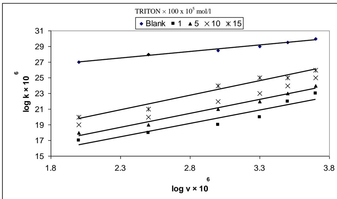
**Figure 4.** Effect of H<sub>2</sub> evolution rate on the mass transfer coefficient of different Triton- $\times$ -100 concentrations.
