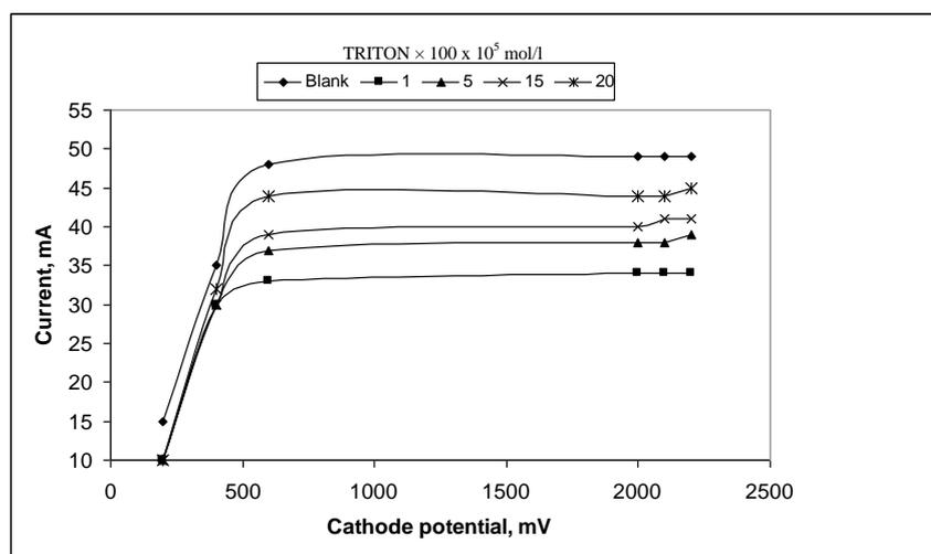
Figure 3. Polarization date in solution containing different Triton-x-100.
