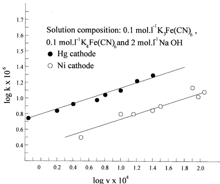
Figure 2. Effect of  $H_2$  discharge velocity on the mass transfer coefficient at Hg and Ni cathodes.
