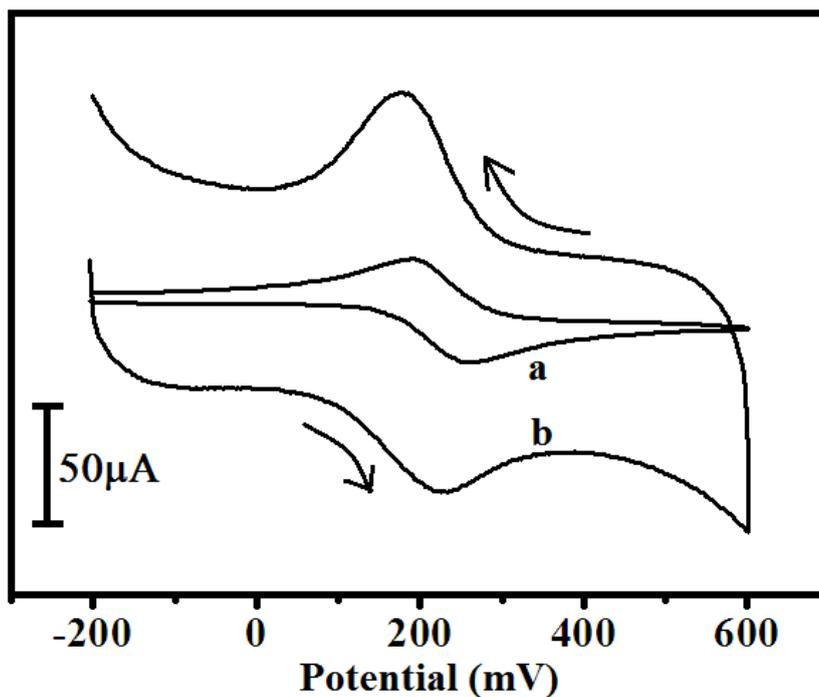
**Figure 1a.** Cyclic voltammograms for the electrochemical responses of  $K_4[Fe(CN)_6]$  at bare (dotted line) and TTABMCPE (solid line) in 1 M KCl containing 1mM  $K_4[Fe(CN)_6]$  at scan rate 50  $mVs^{-1}$ .
