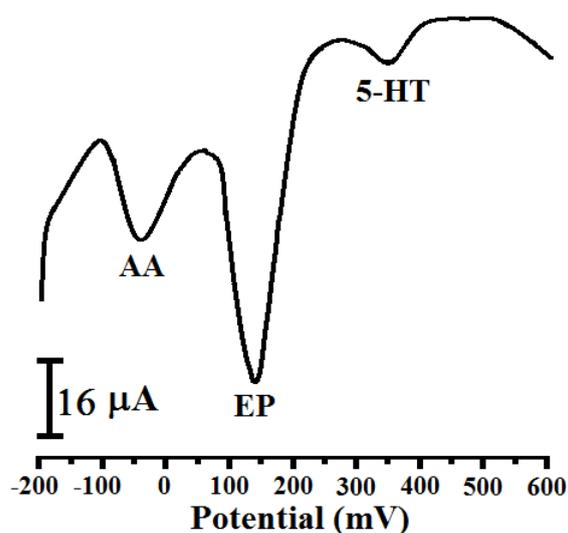
**Figure 10b.** DPV for 1 mM AA, 10  $\mu\text{M}$  EP and 100  $\mu\text{M}$  5-HT at the TTABMCPE in PBS solution at pH 7.4, with a 20  $\text{mVs}^{-1}$  scan rate, 50 mV pulse amplitude, and 50 ms pulse width.
