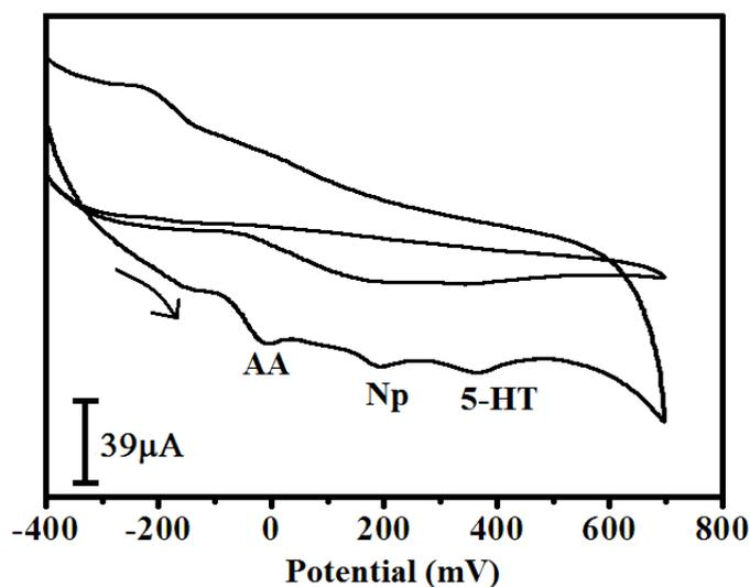
**Figure 10a.** CVs at BCPE (a) and TTABMCPE (b) in 0.2 M PBS (pH 7.4) containing 1 mM AA, 10  $\mu\text{M}$  EP and 100  $\mu\text{M}$  5-HT. Scan rate: 50  $\text{mVs}^{-1}$ .
