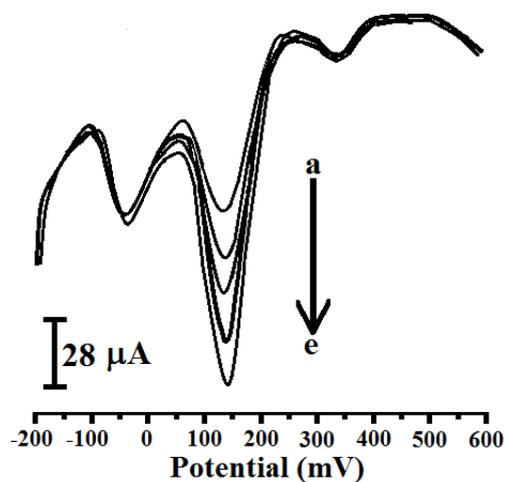
**Figure 11b.** Differential pulse voltammograms of AA in the presence of 10  $\mu$ M EP and 100  $\mu$ M 5-HT in 0.2 M PBS (pH 7.4). AA concentrations (from a to d) [AA]: 1, 2, 3, and 4 mM.
