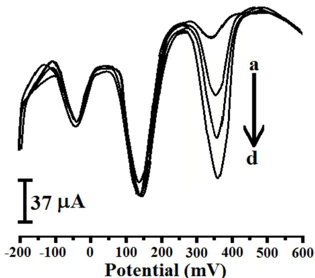
**Figure 11c.** Differential pulse voltammograms of 100  $\mu\text{M}$  5-HT in the presence of 10  $\mu\text{M}$  EP and 1 mM AA in 0.2 M PBS (pH 7.4). 5-HT concentrations from (a to d) [5-HT]: 100,110,120 and 130  $\mu\text{M}$ .
