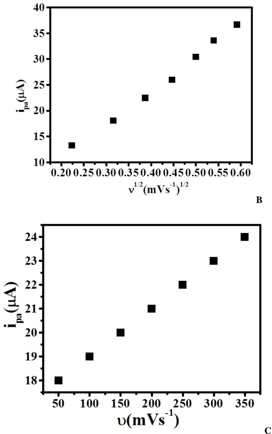
**Figure 5.** (a) Cyclic voltammograms of 10  $\mu M$  EP on the TTABMCPE at different scan rates (a–g: 50, 100, 150, 200, 250, 300, 350  $mVs^{-1}$ ) in 0.2 M PBS of pH 7.4, (b) is the plot of the redox peak current versus the scan rate and (c) is the plot of the redox peak current versus the square root of scan rate.
