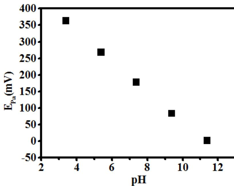
**Figure 7a.** Relationship of  $E_{pa}$  with different pH values of PBS at a scan rate of  $50 \text{ mVs}^{-1}$ .
