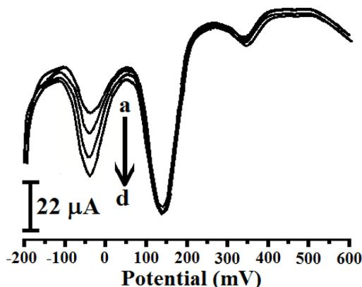
**Figure 11a.** Differential pulse voltammograms of EP in the presence of 1mM AA and 100  $\mu$ M 5-HT in 0.2 M PBS (pH 7.4). DA concentrations (from a to e); [EP] 10,12,14,18 and 20  $\mu$ M.
