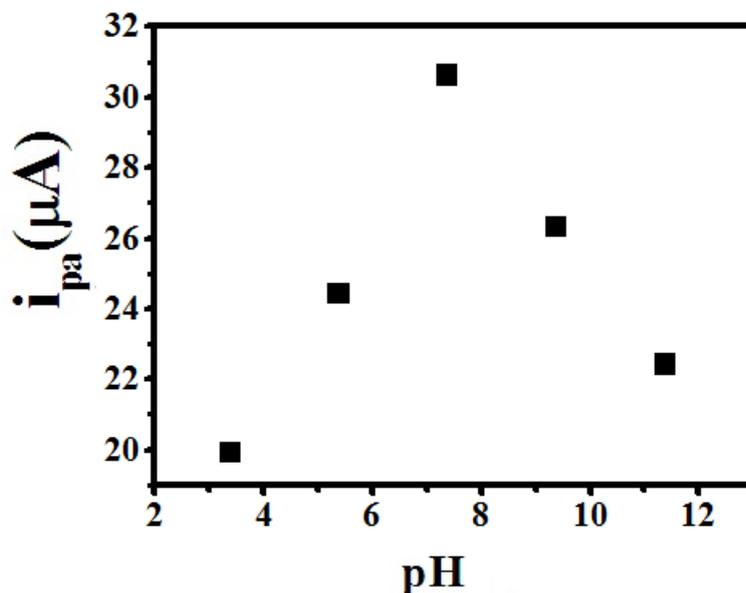
Figure 7b. Plot of  $i_{pa}$  with different pH values of PBS at scan rate of  $50 \text{ mVs}^{-1}$ .
