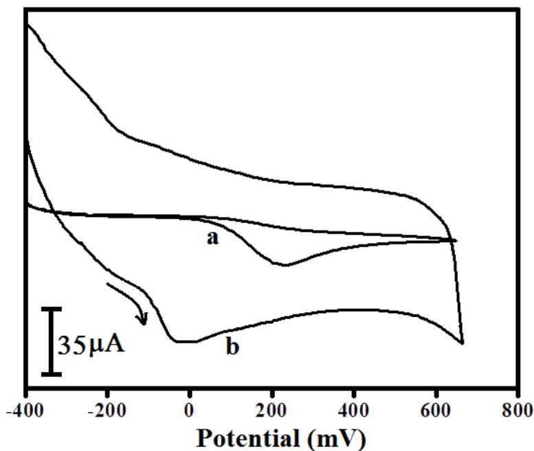
**Figure 9.** Cyclic voltammograms of 1.0 mM AA at a BCPE (a) at a TTABMCPE (b) in pH 7.4 PBS at scan rate of 50  $\text{mV s}^{-1}$ .
