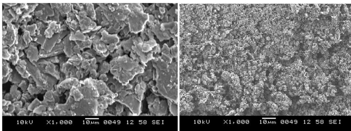
**Figure 3.** Scanning electron microscopic image of BCPE (A) and TTABMCPE (B).
