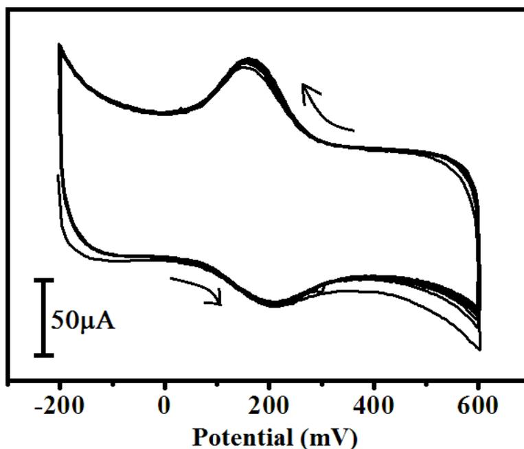
**Figure 1b.** Cyclic voltammograms for 20 multiple cycles of 1mM  $K_4[Fe(CN)_6]$  at TTABMCPE in 0.2 M KCl solution at scan rate of 50  $mVs^{-1}$ .
