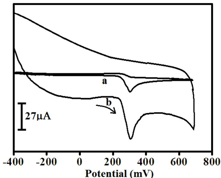
Figure 8. CVs of for  $100 \mu M$  5-HT at BCPE (a) and at TTABMCPE (b) in PBS of pH 7.4 at sweep rate of  $50 \text{ mVs}^{-1}$ .
