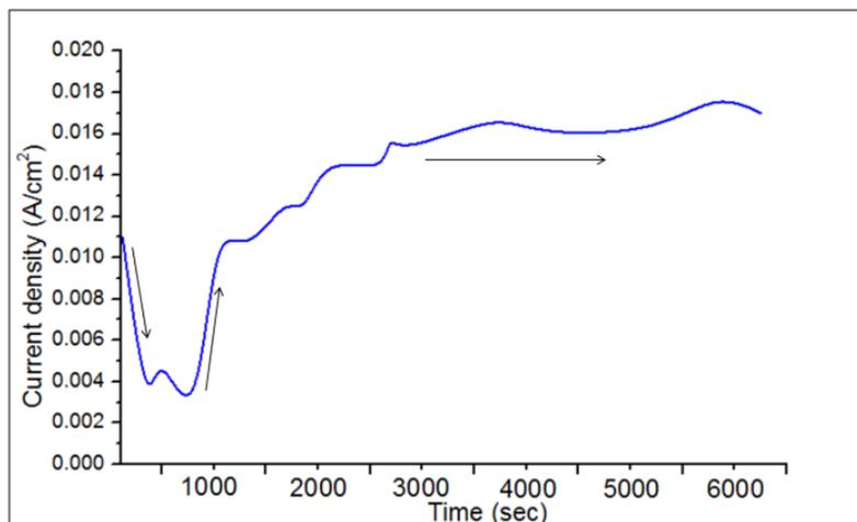
**Figure 4.** current density variation versus time during the electrodeposition of Cu nanowires
