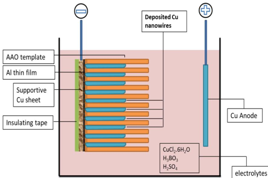
**Figure 1.** schematic diagram of electrodeposition bath for Cu nanowires
