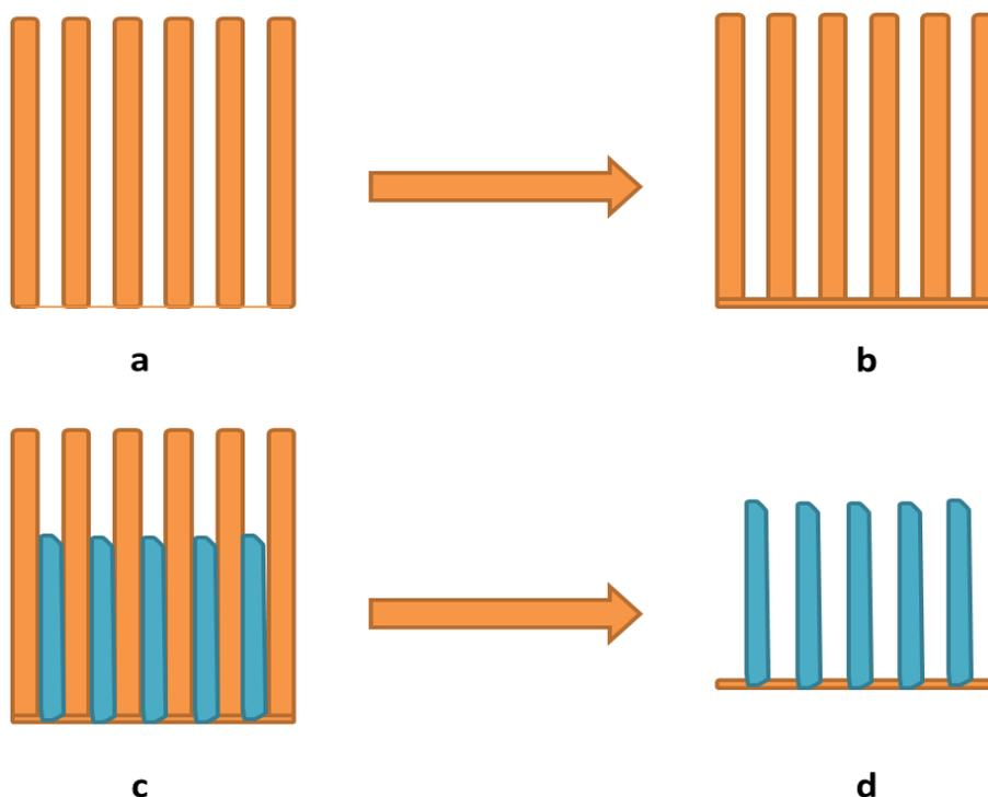
**Figure 3.** A schematic diagram of template filling and removal process; (a) AAO template (b) thin film coated AAO template (c) electrodeposition of AAO template (d) free nanowires after removal of AAO template
