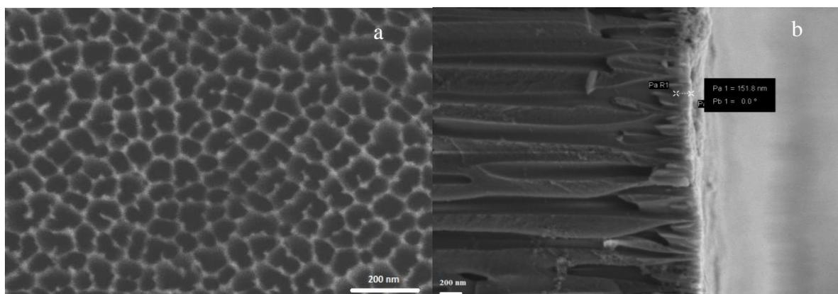
**Figure 2.** (a, b). (a) SEM images of AAO template before deposition (b) thickness of deposited aluminium thin film
