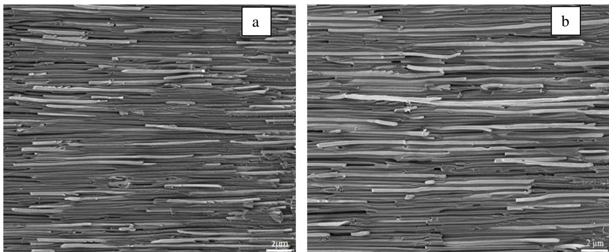
**Figure 5.** (a, b). SEM image of electrodeposited Cu nanowires
