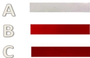
**Scheme 1.** Photos of the prepared sheets of Polymethyl methacrylate (PMMA): (A) blank sheet (B) doped by nap (C) doped by nap-CLA
