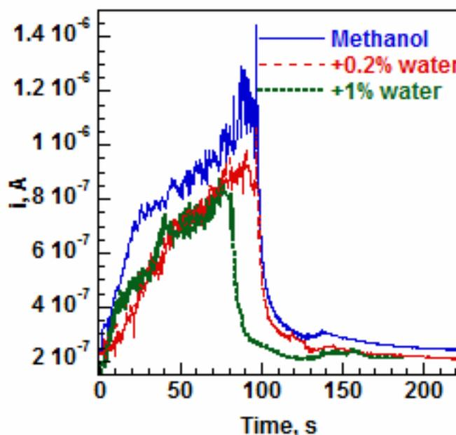
**Figure 3.** Current-time curves of titanium during scratching in methanol solution with different water content.
