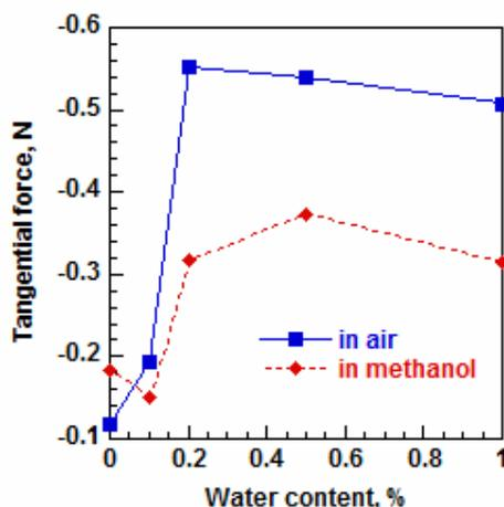
Figure 2. The critical tangential force of the passive film vs. water content.
