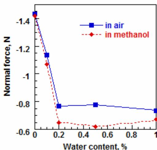
Figure 1. The critical normal force of the passive film vs. water content.
