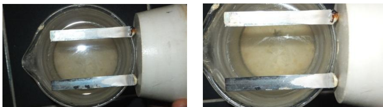
Figure 15. Displays the welded area of the cell with calcium hydroxide. No corrosion products are perceived in the welded joint.
