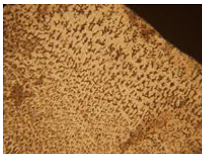
Figure 13. Microstructure with FA (ferritic-austenitic) type dendritic solidification, with not well-defined defined small dendrites. Photomicrograph taken at 20x.
