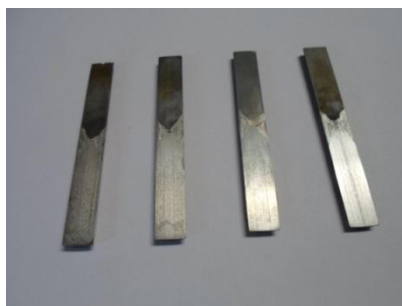
Figure 5. Specimens chemically attacked. The dark zone shows the carbon steel A615, the clear zone shows the stainless steel AISI 304.
