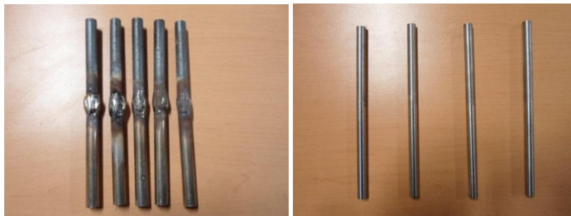
Figure 3. Specimens obtaining Welding process and sharpening of the stainless steel and carbon steel bars.
