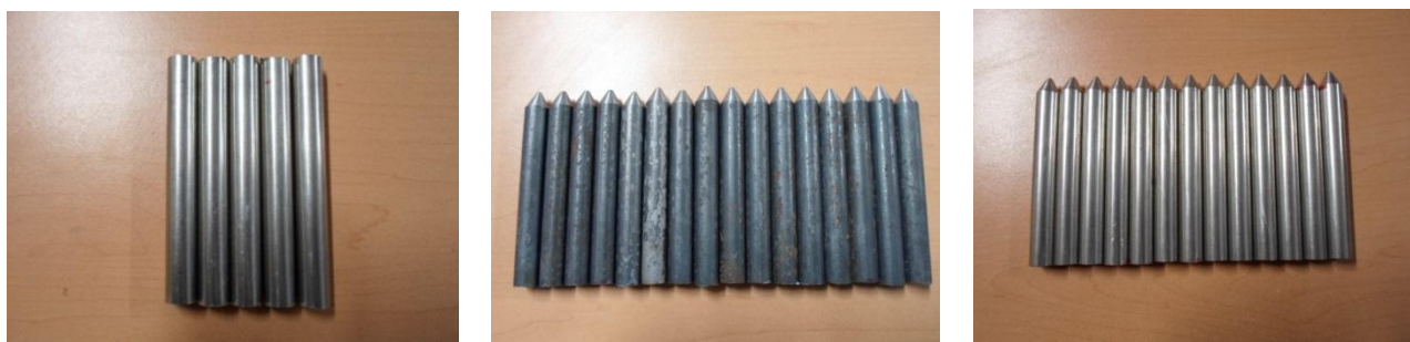
Figure 2. Stainless steel and carbon steel bars with an initial length of 100 mm and Ø = 12.7 mm and after manufacturing the 30 ° bevel pencil tip type
