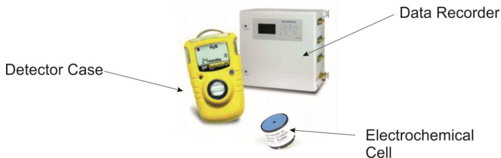
Figure 2. Electrochemical gas sensors produced by Honeywell Analytics ( www.honeywell.com ). A electrochemical cell consists of electrodes, membrane and insulate separators (to keep electrodes away from each other). A detector case has a complete electronic circuit which allows the gas concentration to be read. A data recorder can continuously record the gas concentrations.
