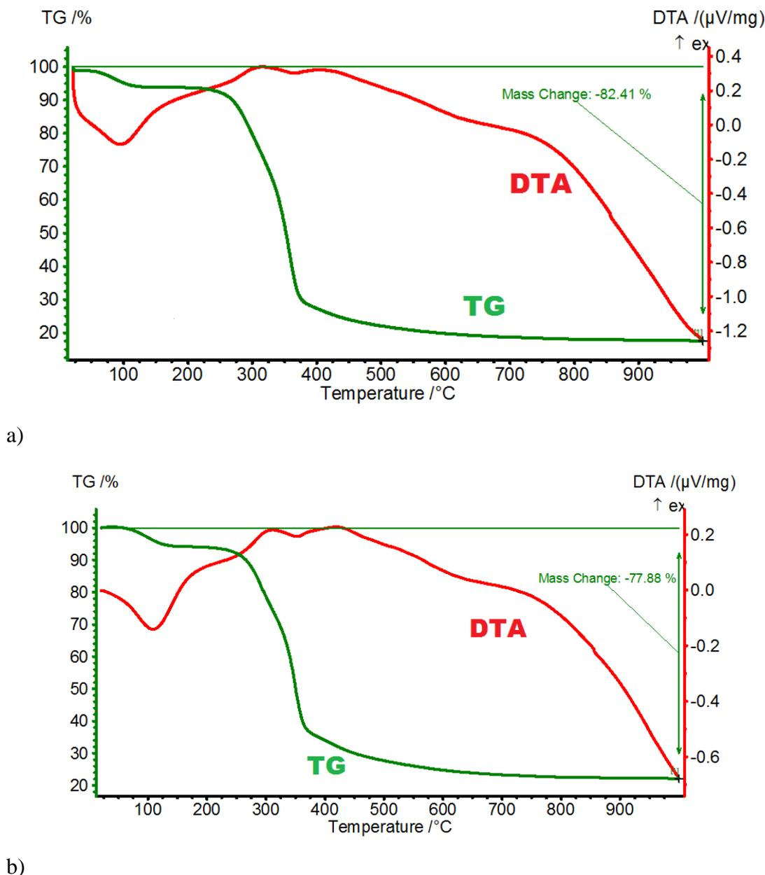
**Figure 5.** The DTA-TG curves recorded for carbon-based fuels originating from beech wood (a) and acacia wood (b)
