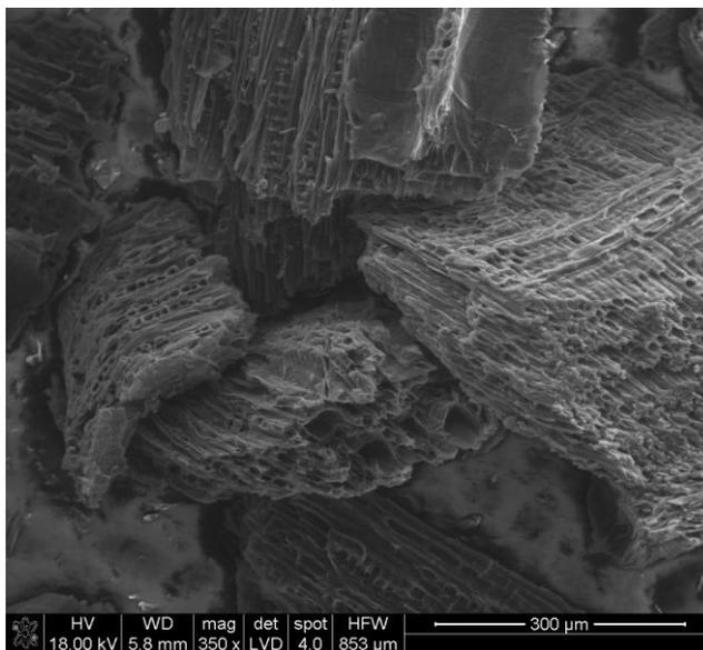
**Figure 6a.** SEM microscopy of carbon particles originating from raw beech wood (A) during DC-SOFC operation.
