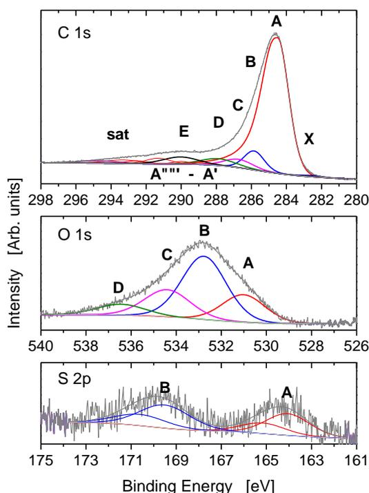
**Figure 4.** The deconvolution of C 1s (a) , O 1s (b) and S 2p (c) core excitations.
