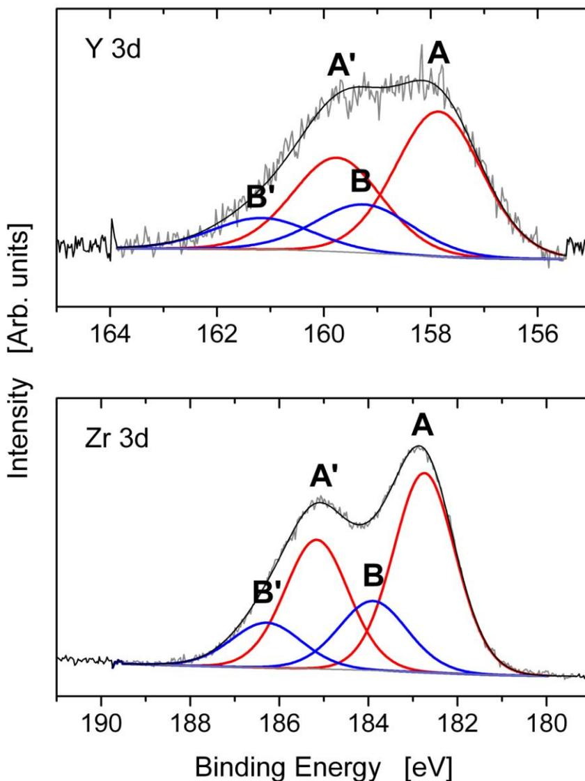
**Figure 7.** The deconvolution of Y, Zr core excitations.
