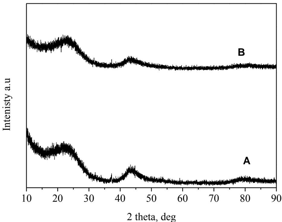
**Figure 2.** The XRD diffraction pattern recorded for carbon-based fuels originating from beech wood (A) or acacia wood (B)
