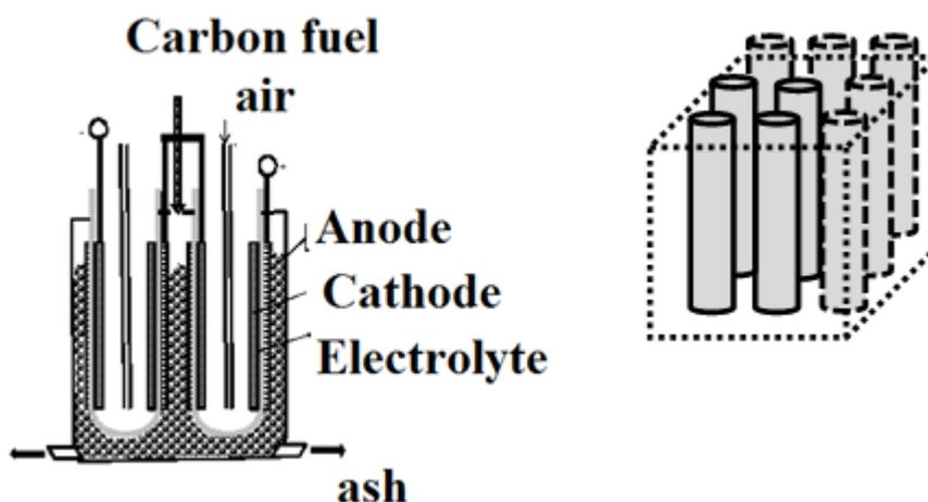
**Figure 11.** The proposal of construction of the short tubular solid oxide fuel cell stack fed with biochar
