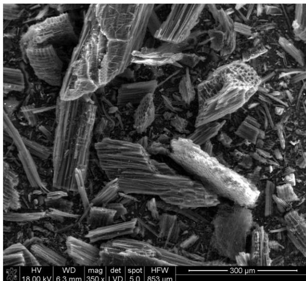
**Figure 6b.** SEM microscopy of carbon particles originating from raw acacia wood (B) during DC-SOFC operation
