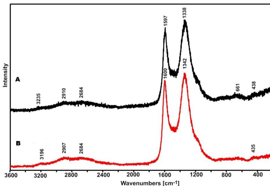
**Figure 3.** Raman spectra recorded for carbon-based fuels originating from beech wood (A) or acacia wood (B)
