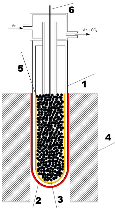
**Figure 1.** The tubular direct carbon solid oxide fuel cell: 1- Electrolyte 8YSZ, 2- cathode LSM, 3- Ni-GDC, cermet anode material, 4 – electric furnace, 5 – solid fuel
