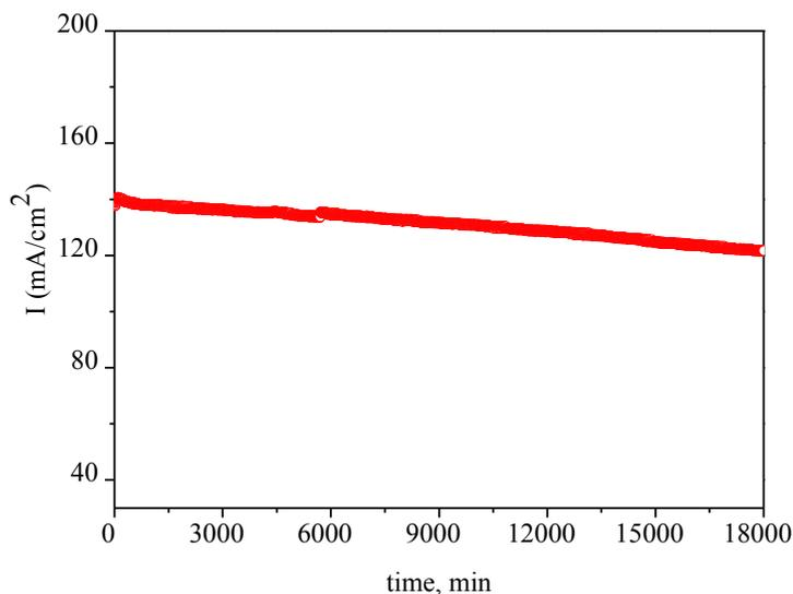
**Figure 10.** The TDC-SOFC operation under load  $\Delta E = -0.5V$  at  $800^{\circ}C$ . The raw beech chips were used as fuel
