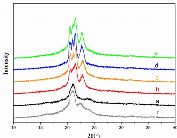
**Figure 6.** XRD patterns of the PBC nanofiber films (r: raw material, a: just prepared, b: 1 day after prepared, c: 2 days, d: 4 days, e: 10 days)
