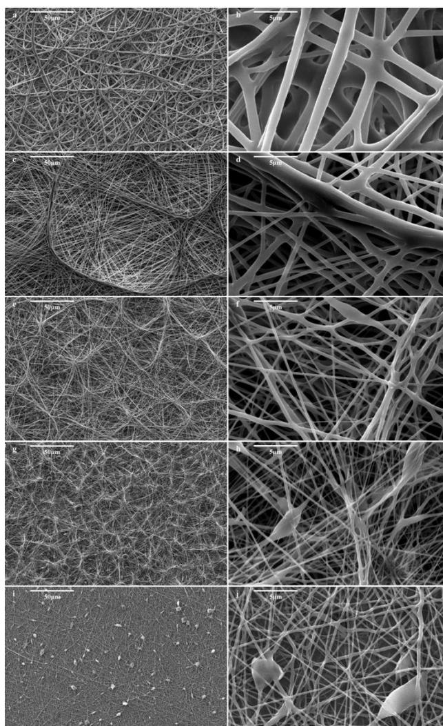
**Figure 4.** Scanning electron micrographs of PBC nanofibers prepared from  $\text{CHCl}_3$ -DMF mixed solvents(a,b-8:2, c,d-7:3, e,f-5:5, g,h-3:7, i,j-2:8).
