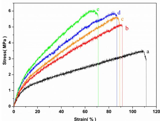
**Figure 7.** Strain-Stress curve of the PBC nanofiber films (a: tested that right day, b: 1 day after prepared, c: 2 days, d: 4 days, e: 10 days)
