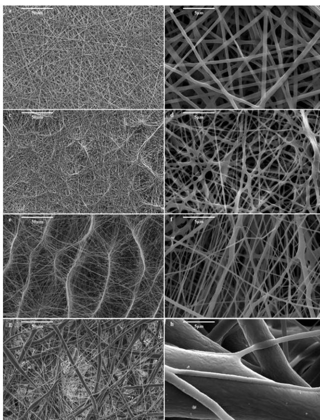
**Figure 3.** Scanning electron micrographs of PBC nanofibers prepared from single solvents (a-b: FA, c-d: DMF, e-f: HFIP, g-h:  $\text{CHCl}_3$ ).
