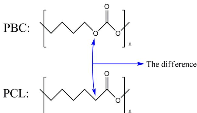
**Figure 1.** Structure of PBC and PCL
