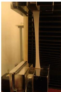
**Figure 2.** showed a photo taken from the tensile test.
